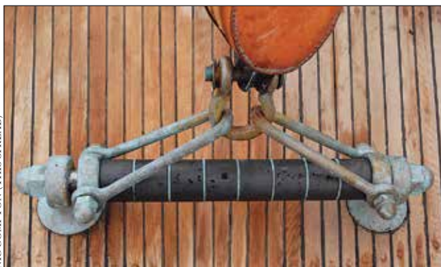
All of INTEGRITY's hardware, including this mainsheet horse, was cast by Major Castings in Fowey, which also welded the copper stemband that appears on the facing page.
