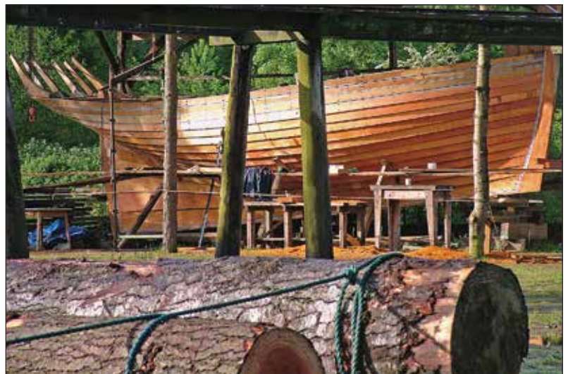
ALERT's lapstrake planking is traditional for the smuggling cutter type, and it sets the boat apart from several other recently built British cutters, which were planked carvel-fashion.
