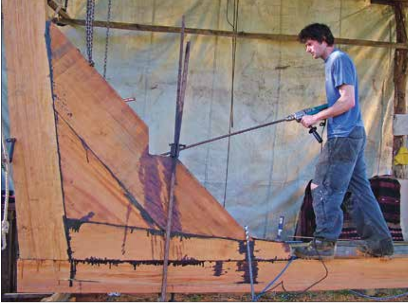
To build ALERT, Stirling worked 15 hours per day, six days a week, for a year and a half. Here he is boring the cutter's shaftlog.
